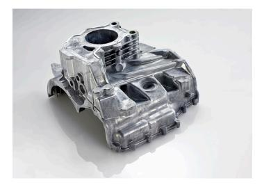
Test sample – Casting condition after S&E treatment.
